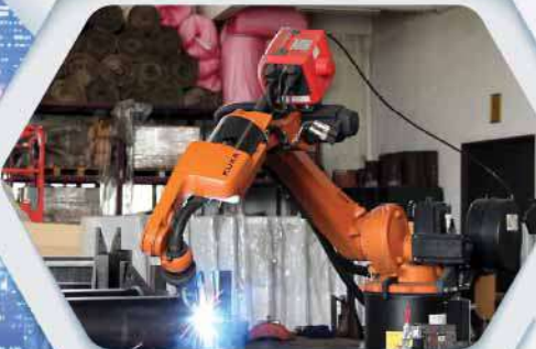
Robotic Welding Machine
